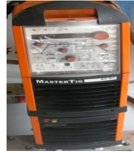
FIGURE 4. 3500-watt AC/DC Gas Tungsten Arc welding machine
