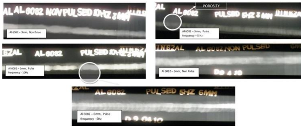
FIGURE 6. Al 6082 welded samples – Pictures of Radiographic Test
